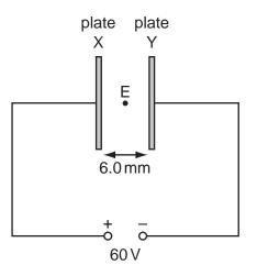
What is the electric field strength at E, a point midway between the plates?
