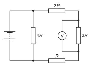
The voltmeter reading is 2V.
